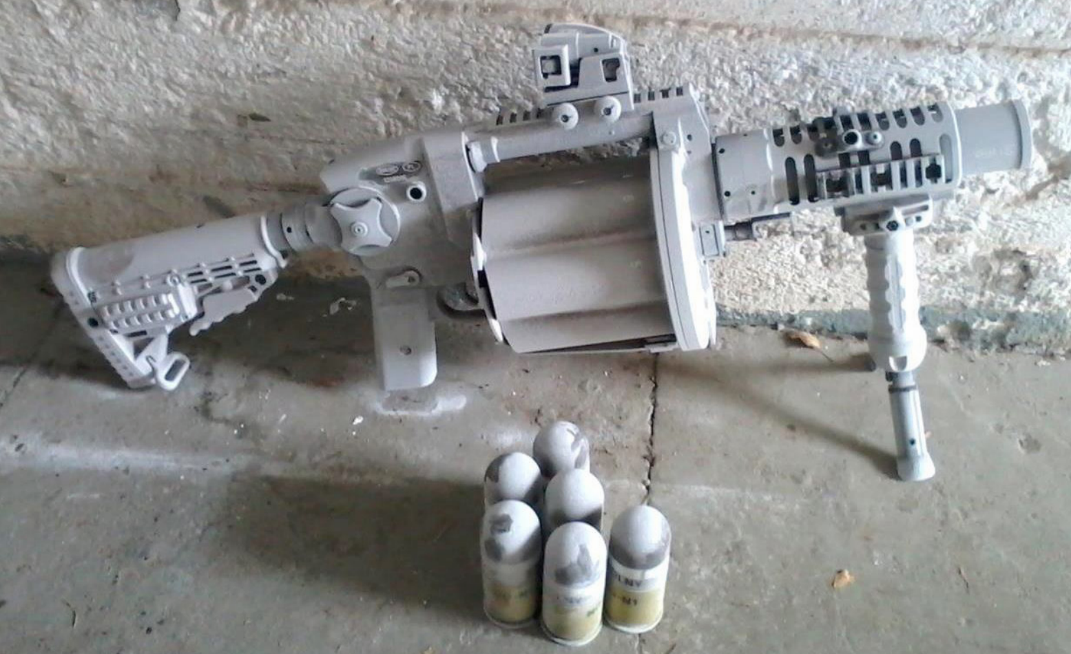
▲ Dust and sand tests at +55°C
