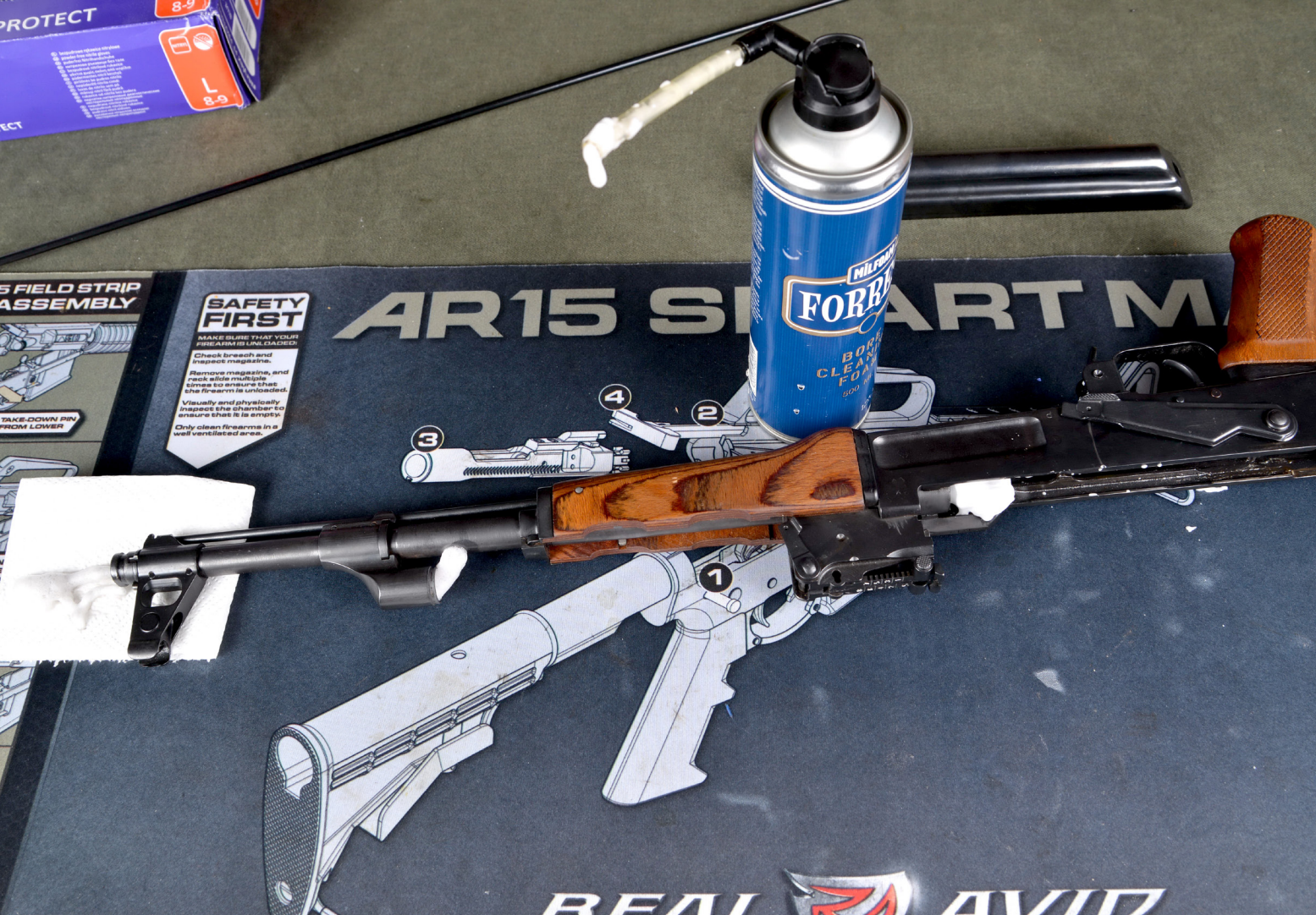
▲ Rifle with foam injected into the barrel and set aside until the chemical softens the residue
