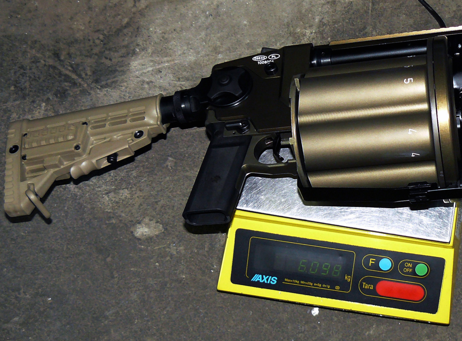
▲ RGP-40 with titanium elements and without the sights and front grip/bipod assembly massed at 6.098 kg. This increases to 6.361 kg with the grip/bipod mounted
