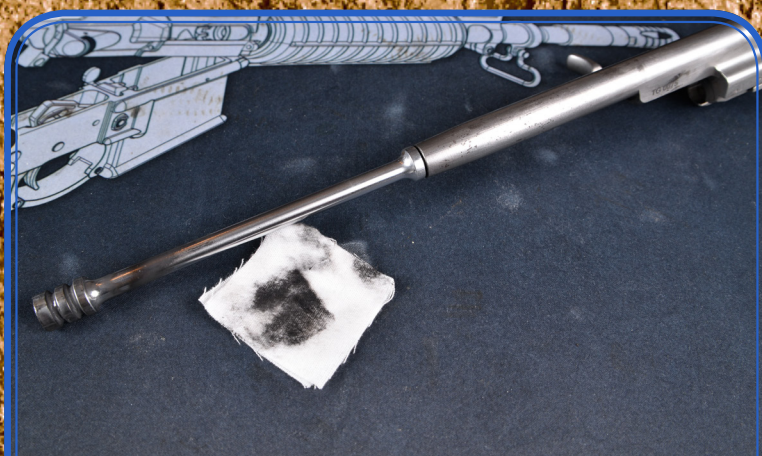
▲ Just wiping with a cotton cloth before using chemistry removes a lot of residue
