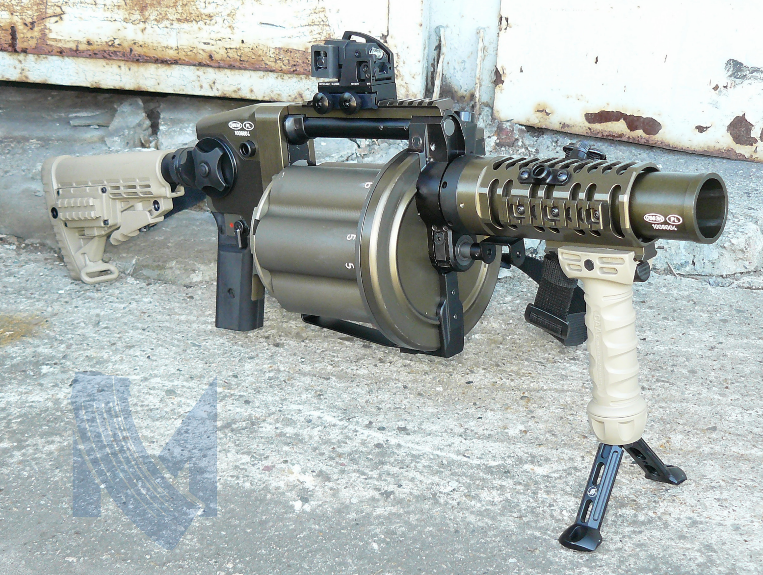
▲ RGP-40 from the test batch. One of these had titanium alloy elements. The other had it's mass reduced by cut-outs and material removal
