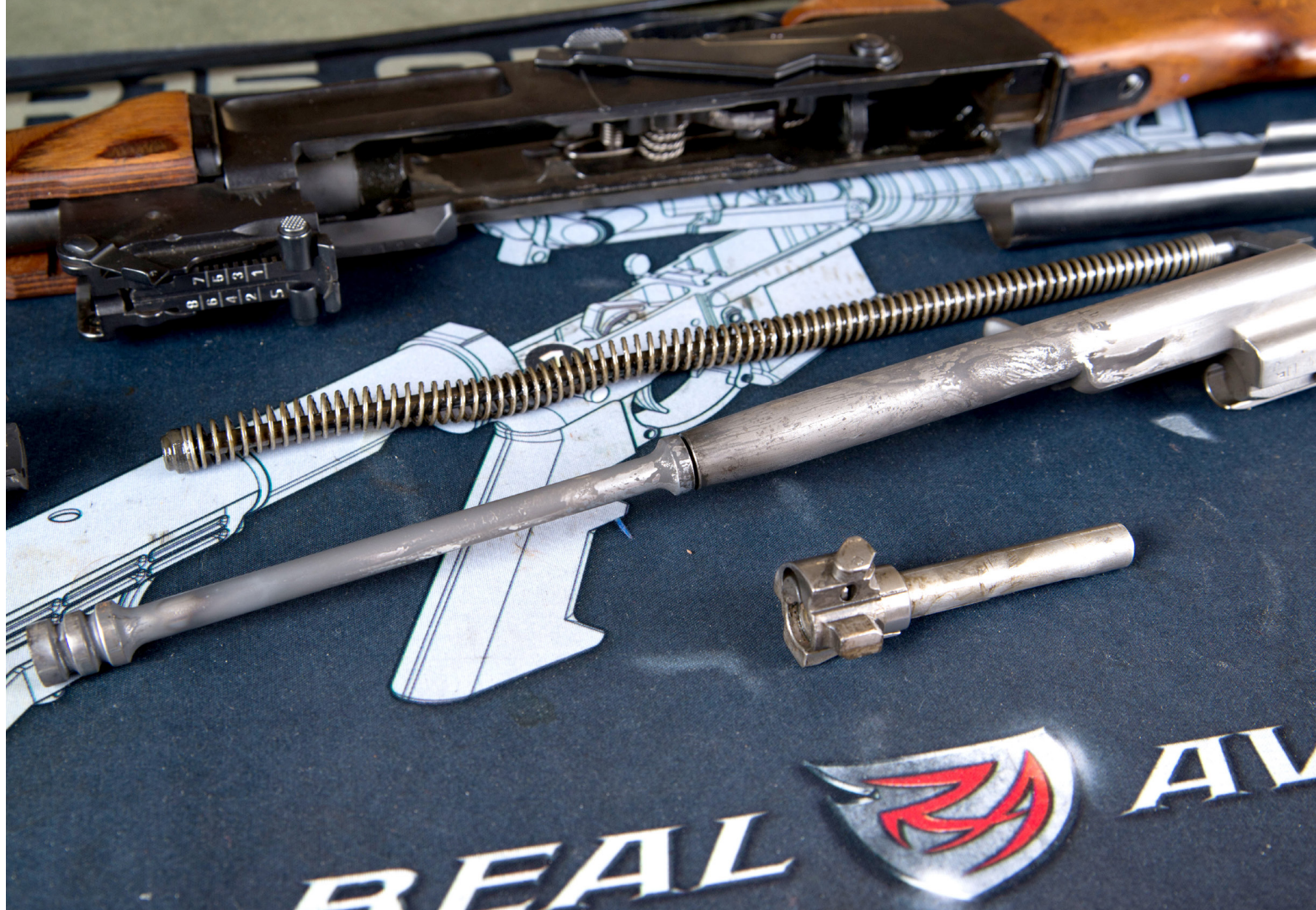
▲ AK bolt carrier and chamber before cleaning, after firing about 50 rounds
