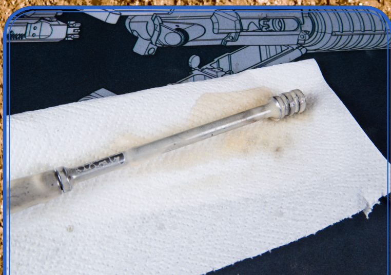
▲ AK bolt carrier before cleaning, after firing about 50 cartridges
