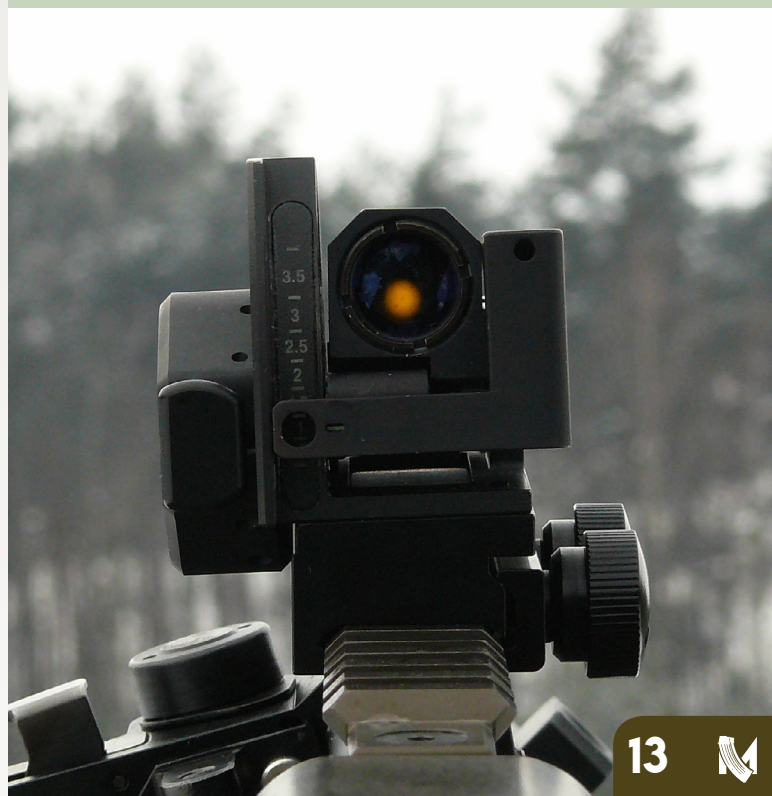
▼ First models and prototyped utilized Israeli made Meprolight GLS-203 reflex sight with an orange dot
