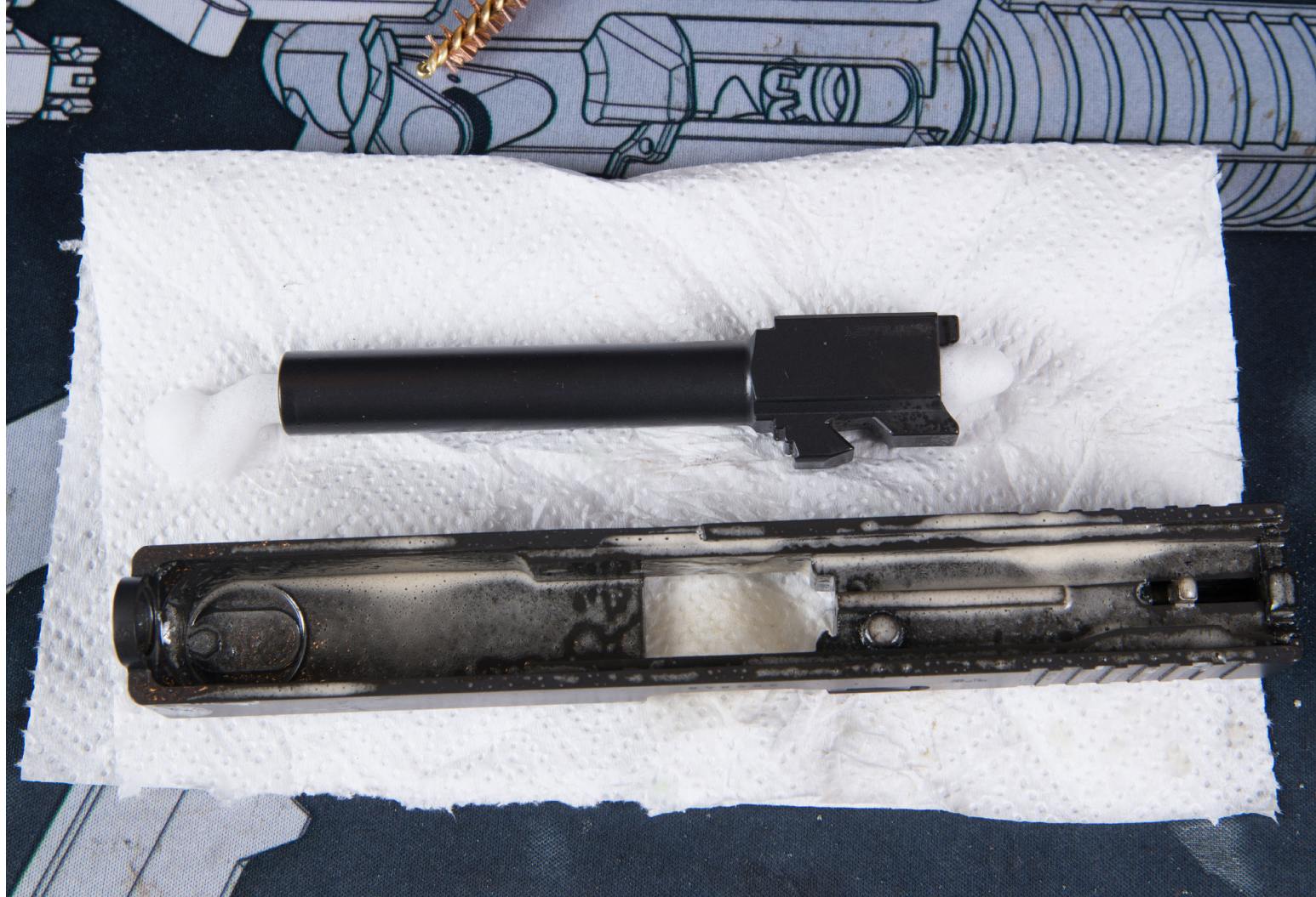
▲ The cartridge chamber and the lock were treated respectively with foam and cleaning agent
