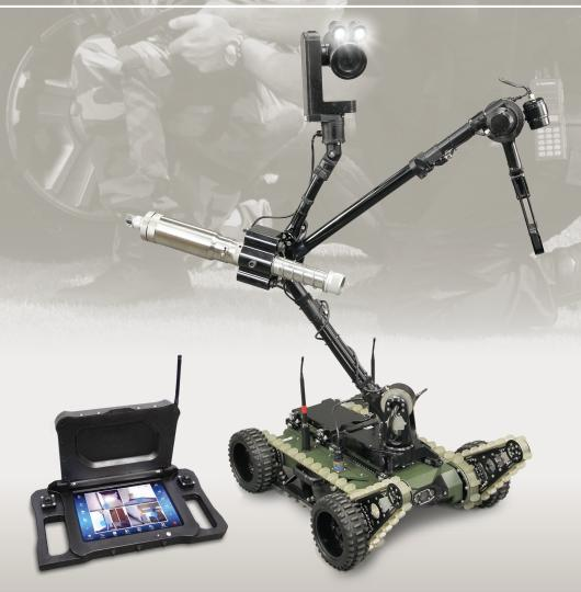
PIAP GRYF® is a robot used for reconnaissance of terrain and hard to reach places. The manipulator with 5 degrees of freedom allows to lift loads weighing up to 15 kg.
