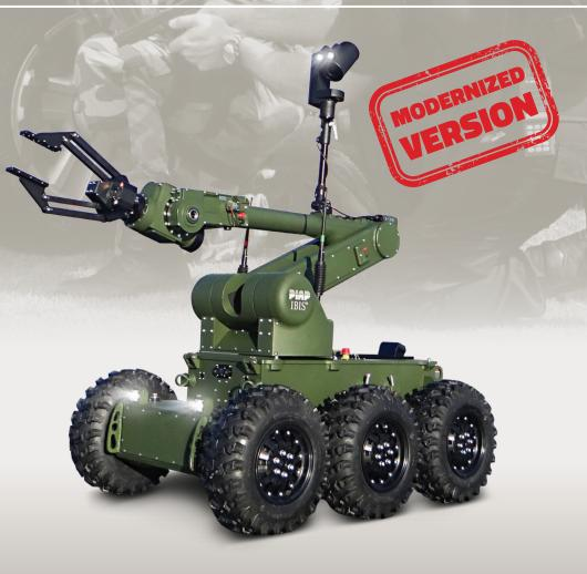
IBIS® is a robot for pyrotechnic operations and reconnaissance. Upon installation of additional devices, it can be used, among others, for disposal of dangerous objects, chemical detection and rescue operations. Six-wheeled chassis with independent drive of each wheel allows to operate in challenging and varied terrain (bedrock, wetlands, muddy terrain and debris).
