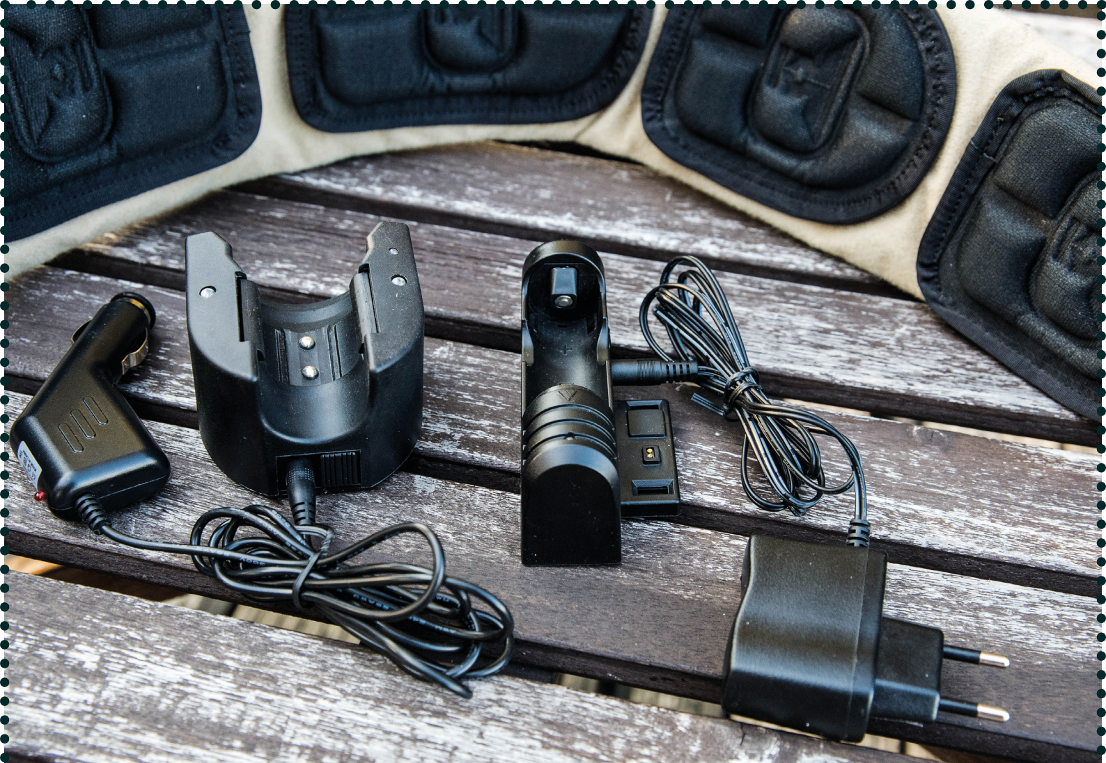
Docking station and battery charger can be used separately. Each has two power sockets, traditional and micro USB
