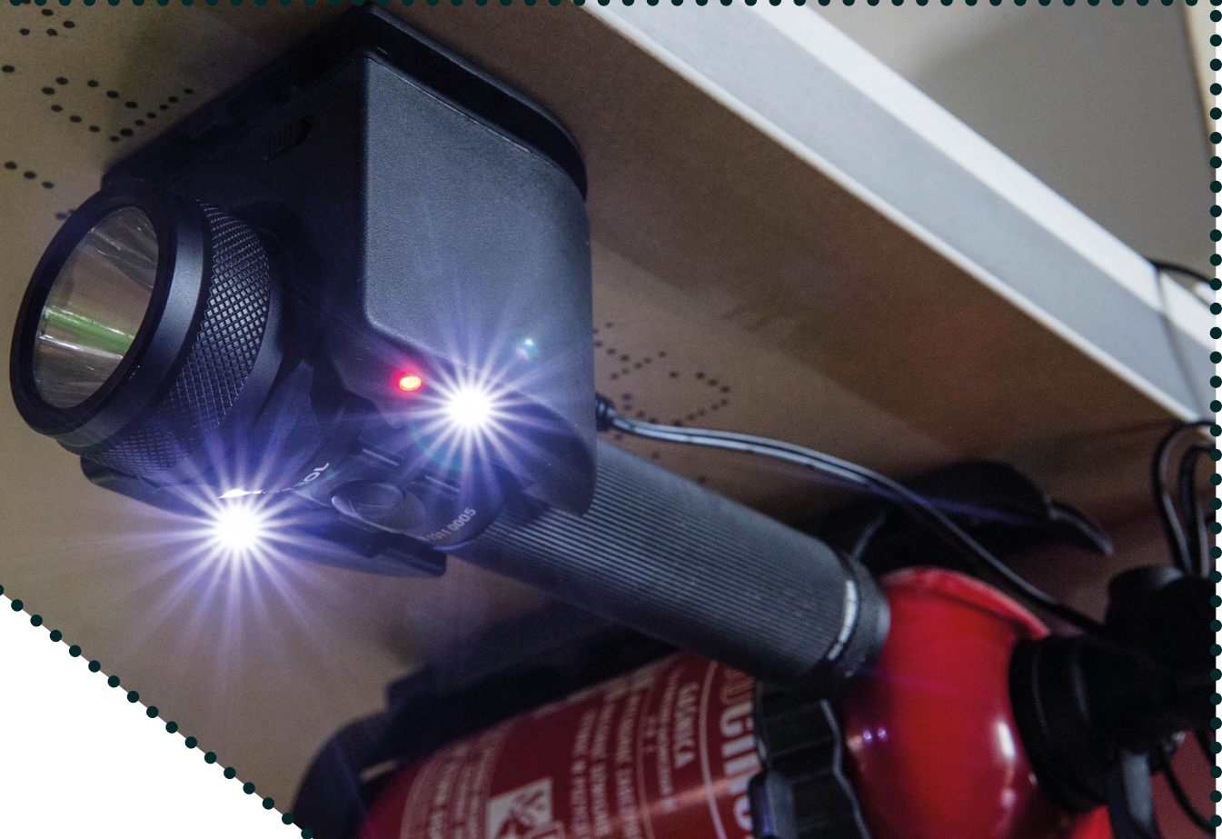
The station installed at home underneath the countertop. Lit up dock works finely during the power outage
