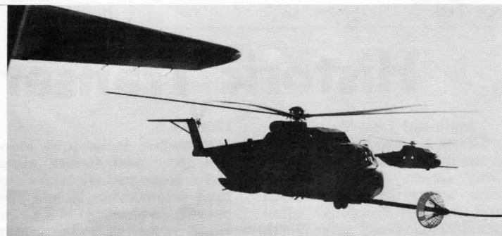
HH-3E refuels in flight from an HH-130 tanker airplane over Scotland on the final leg of the transatlantic flight. Both HH-3Es were refueled a total of 18 times during the 30 hour, 46 minute flight from New York to Paris.
